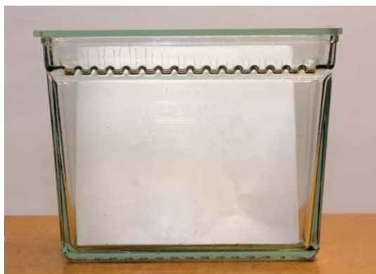
Figure 7.3 Photograph illustrating a chromatography tank used in thin-layer chromatography.
