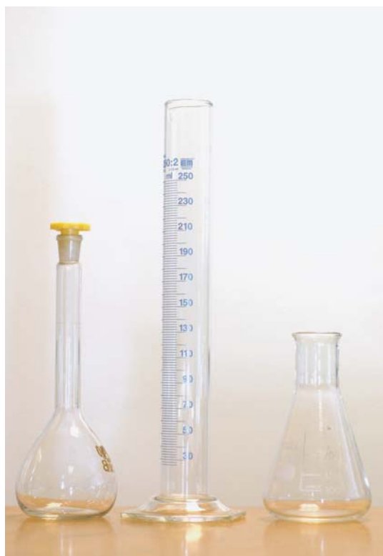
Figure 2.3 Typical pieces of laboratory glassware used in volume measurement.
