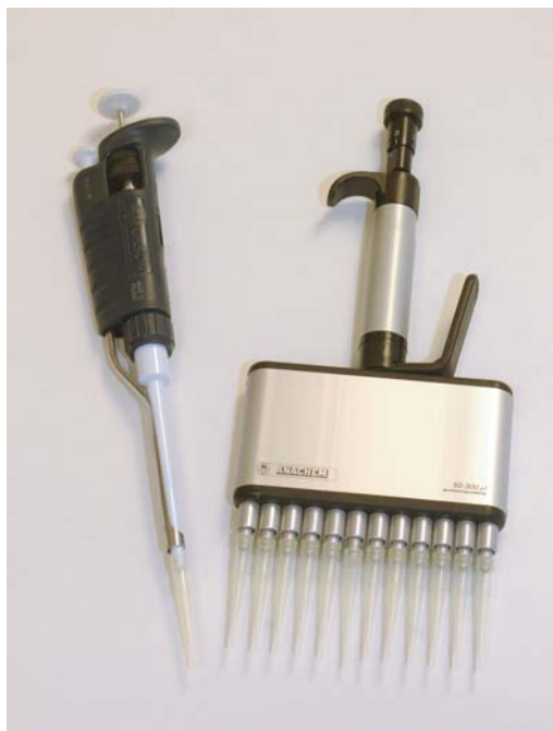
Figure 2.4 Photograph showing a single channel and multichannel Gilson Pipetman.
