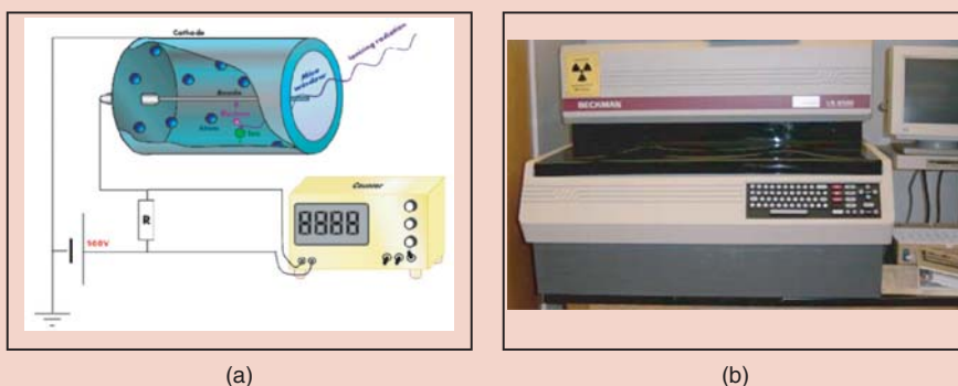
Figure 10.5 Diagram of a Geiger–Müller tube (a) and photograph of a liquid scintillation counter (b).
