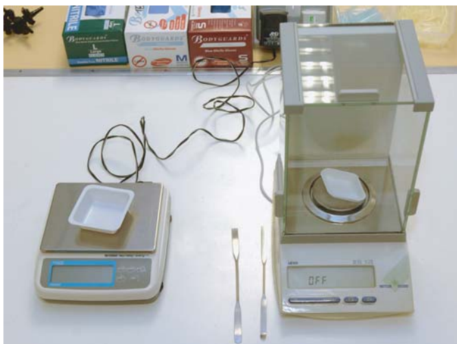
Figure 2.2 Photograph illustrating typical laboratory balances and weighing equipment.
